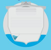
Waste water captured in machine spaces that contains small amounts of oil or other contaminants resulting from normal operation and routine maintenance.
